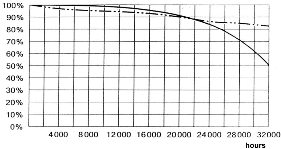
Drawing 2. Operational curves of changes of the luminous flux of high pressure sodium lamps with the power of 150 W, type NAV 4Y
